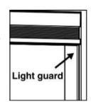
b. When light guard length > shade width and  $\geq$  2000mm, light guard will be sliced into 2 parts evenly.
