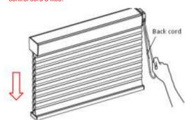
Note: the control cord cannot be too tightened / taut when installing due to its own system character.
