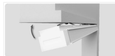
figure 5: rotate the head track until it 'clicks' into the clips
